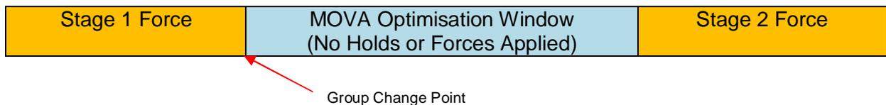
The use of the MOVA Optimisation Window allows the local MOVA controller to find gaps to safely change before moving to the next stage.
