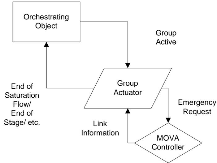
**Figure 2 Relationship between Orchestrating Object, Group Actuator and MOVA Controller**
