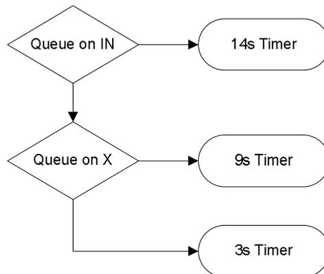
**Figure 4 M271 NB Timer Selection Logic in Group Actuator**
